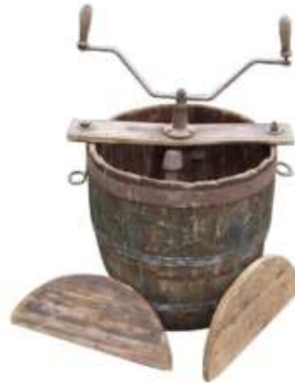
'Back-and-forth' washing machine. This consisted of a barrel in which the three blades were moved from left to right by two people using a flywheel-crank located above the receptacle.
